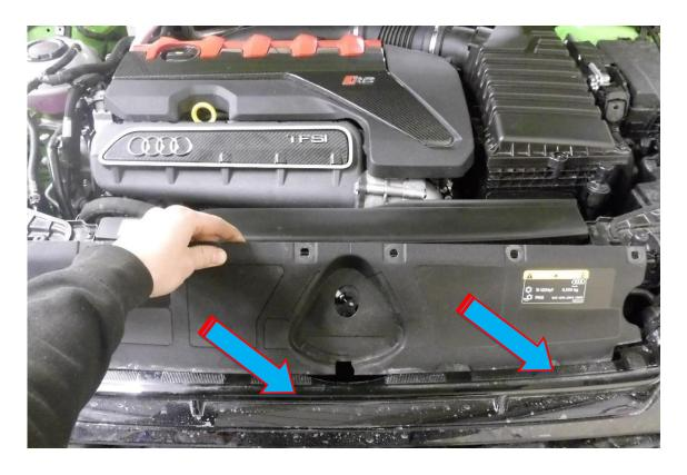
4. Using a T27 Torx drive remove the 3 X fasteners attaching the grill to the vehicle.
