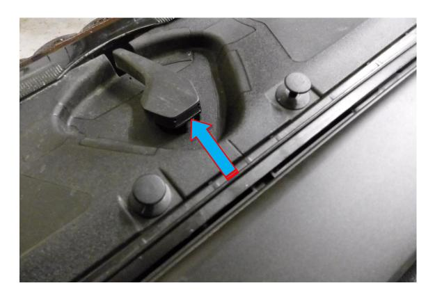
3. Pull the plastic slam panel upwards to remove it.
